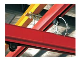
Single-girder suspension cranes from the KBK monorail crane provide a fast and safe area-serving overhead handling solution and exact positioning of a wide variety of goods.
