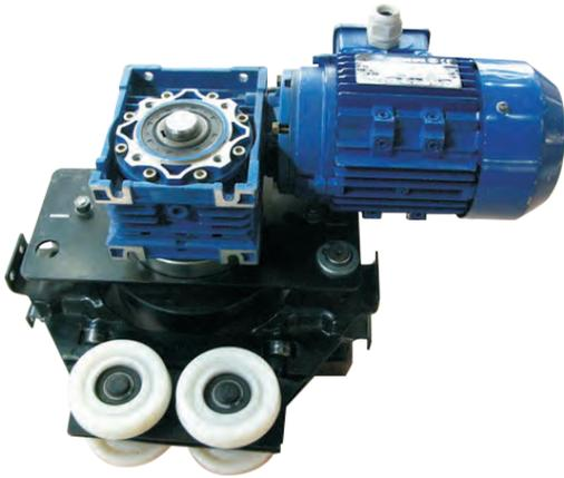
Motorized trolley to drive the hoist and girder.
